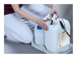
Liquid detergent is automatically dispensed from a canister located close to the dishwasher. The detergent is added to the wash liquor via a dispenser pump and a siphon according to the dispensing concentration selected.
